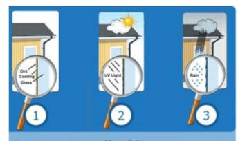
Figure 1: Coating is activated by UV light ter installation the special coating needs 5 to 7 days exposure to daylight to activate fully
